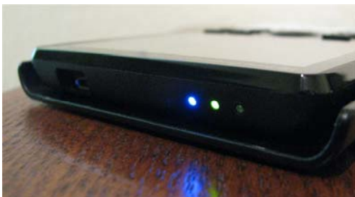
Figure 4 Exam mode lights blinking a unique sequence
