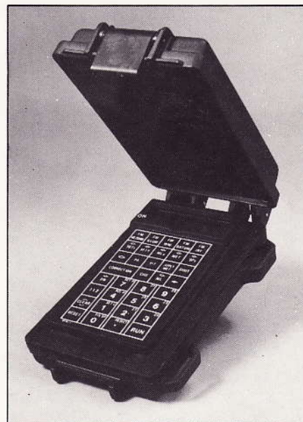
▲ The Morzen mortar fire control computer is housed in a shock- and water-proof casing. Essentially, it is a Hewlett-Packard HP41 hand-held computer
